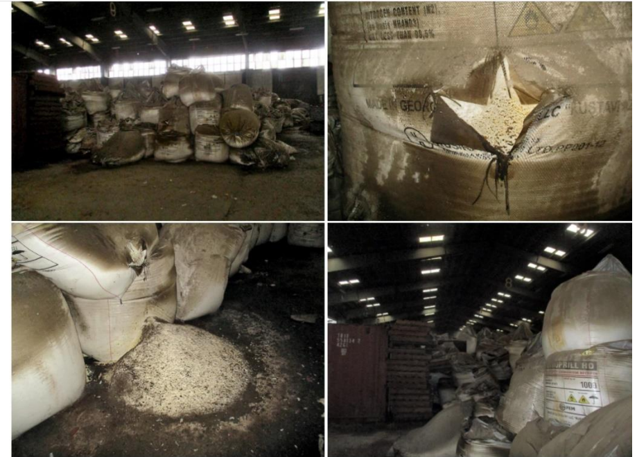
Bags of ammonium nitrate were piled haphazardly in Hangar 12, some torn and spilling their contents. The New York Times
